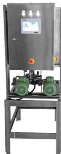
2x50 lpm pump station for greenhouse
